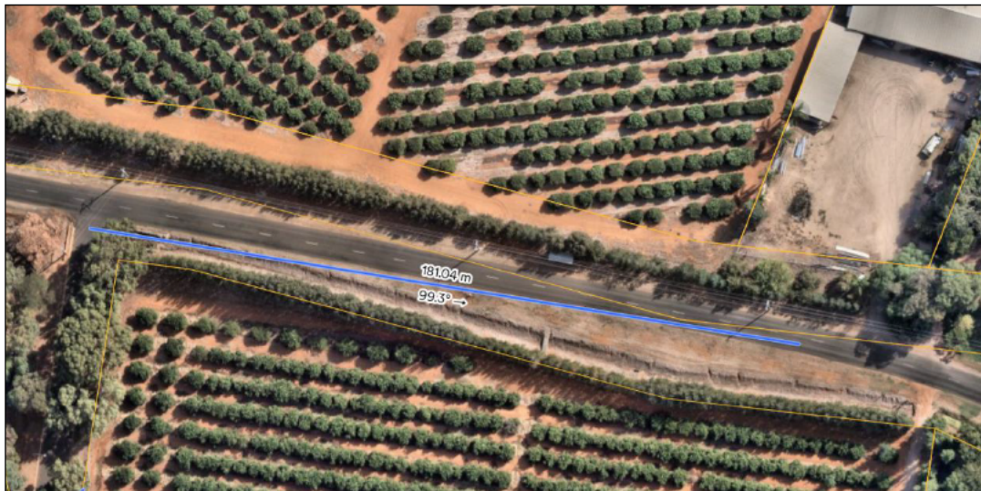
Figure 14: Sight line from Maegraith Place of 181 m to the east along Mallinson Road is satisfied
