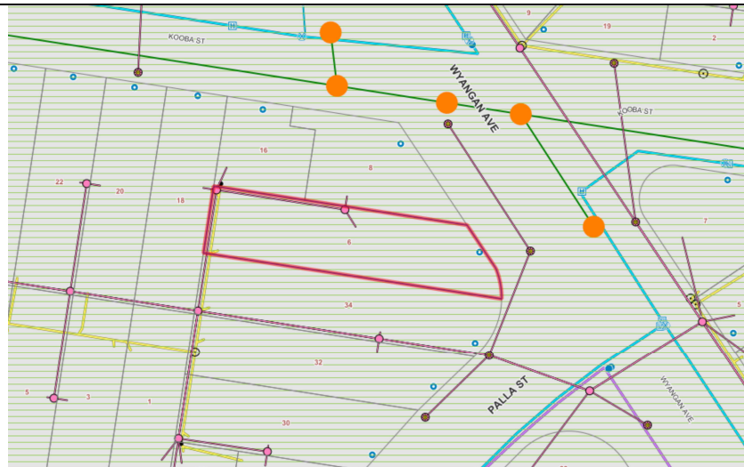
Infrastructure – pink – overhead electricity, dark brown – underground electricity, yellow – sewer, blue – water, green – drainage network
